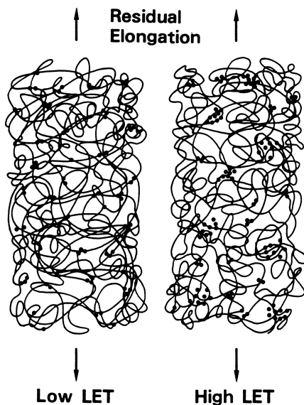
Figure 9. Schematic representation of heterogeneous crosslinking for low and high LET radiations
