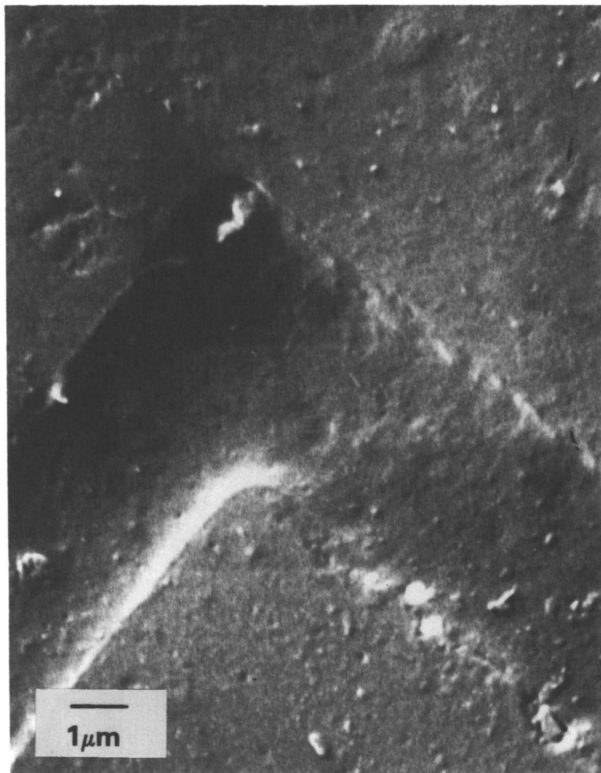
Figure 8. Scanning electron micrograph of a portion of Figure 7. The imperfections are due to the condition of the original PET film and to mask errors.
